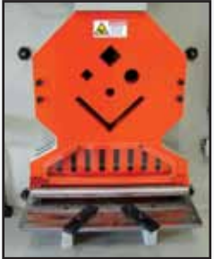
Shearing station with hydraulic hold down
